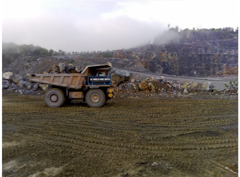
Bi-Fuel (Diesel-LNG) Komatsu 80T Haul Truck
