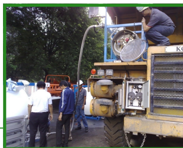
Onsite Refueling with LNG
